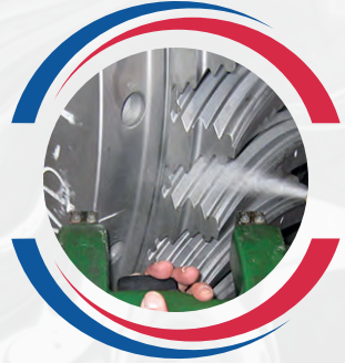
Magnetic Particle Testing (MT)
